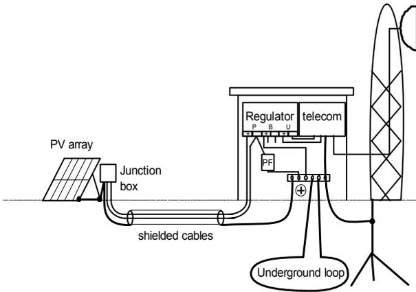
The connection between modules and charge regulator should be shielded. All metal parts should be grounded. Lightning rods can help to protect from voltage spikes but they should not shadow the modules at any time.
