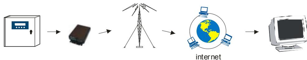
forwarded to a PC via a serial interface (optional USB). The Data collection frequency can be chosen freely to determine the data collection period. An additional analogue input can register external parameters, that cannot be measured by the System-Manager itself: wind speed, module temperature, solar radiation, etc. The logger comes with the necessary software to operate all the above features.
