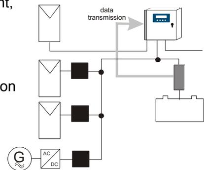
⇒ An external data logger can be connected to the System-Manager. It stores essential system parameters that can be
