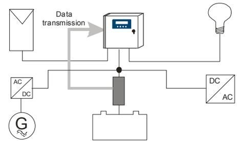
⇒ The included external temperature sensor must be used to tell the PowerTarom the actual battery temperature. The final charge voltage will then be optimized by a temperature compensation.
